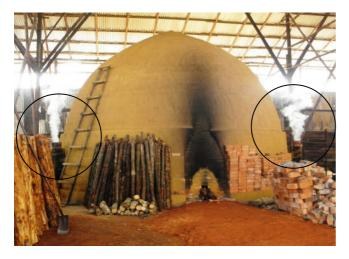
Fig. 1. A dome-shaped charcoal kiln in Matang with smoke emitting from the vents
